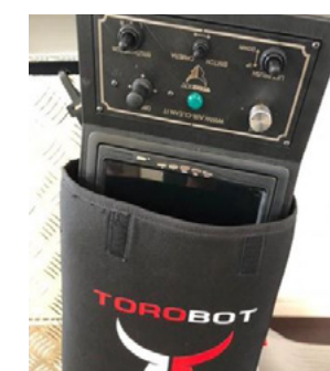
Pocket (customizable) for joystick storage during work session and transport
