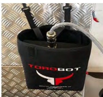
Pocket (customizable) for joystick storage during work session and transport
